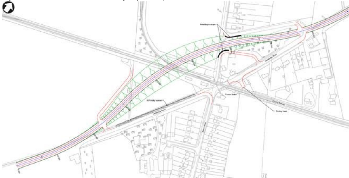
Figure 2: Indicative overbridge option layout from GRIP2 report
